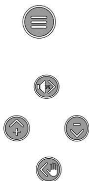
To enter parameter programming, hold the key
