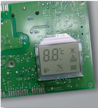
HONEYWELL electronic PCB with microprocessor
